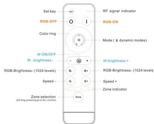
**Note:** Short press "Zone Selection" key, for single zone shift, selected zone indicator lights on. Long press "Zone Selection" key for 2 seconds selects all zones – all indicators light up. All zones are controlled simultaneously.
